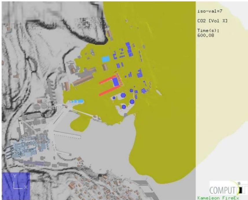
Figure 64 - Release rate of 500 kg/s and directing downwards, windspeed 1 m/s from North
