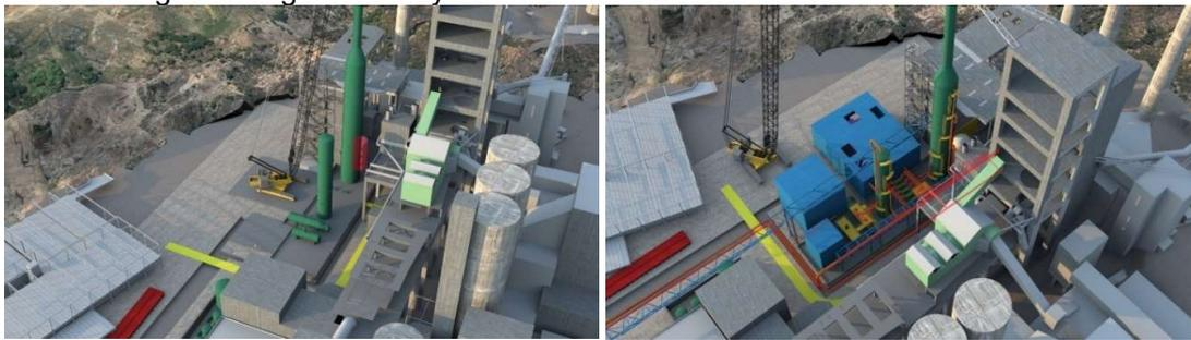
Figure 57 - Location of crane for lifting operations in the main process area
