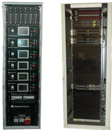
Figure 3-14: AKSO topside cabinet (EPU and Subsea Gateway)
