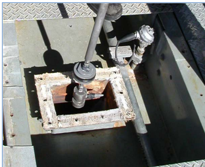
Figure 3.6 In-stack sample probe fitted with a 90 mm stainless steel filter holder
