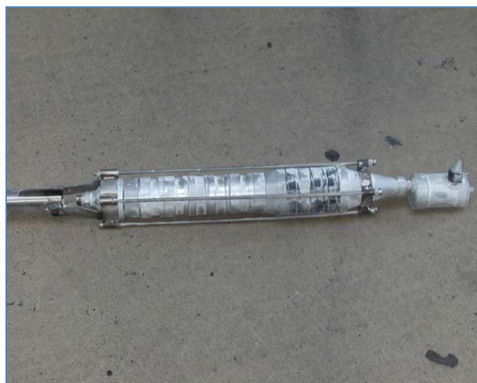
Figure 3.7 In-stack, seven-stage cascade impactor for particulate sampling
