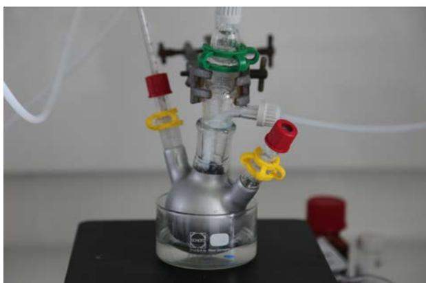
**Figure 3.1.** Picture of the denitrosation reaction vessel.
