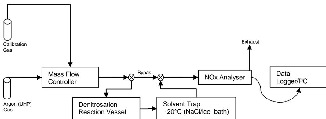
**Figure 3.2.** Schematic of denitrosation apparatus
