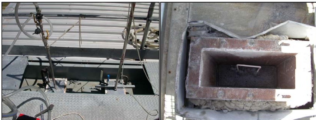
Figure 2.7. Rectangular section sampling ports: (a) sampling probes installed; (b) showing flange fitting to eliminate gas stagnation. (Copyright CSIRO, CCSD 2010)
