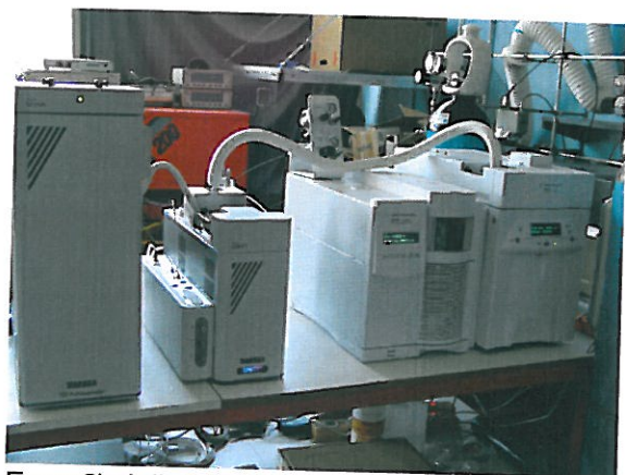
Figure 2b: Agilent Technologies 6850 GC-MS. A direct sampling module is connected in the middle.
