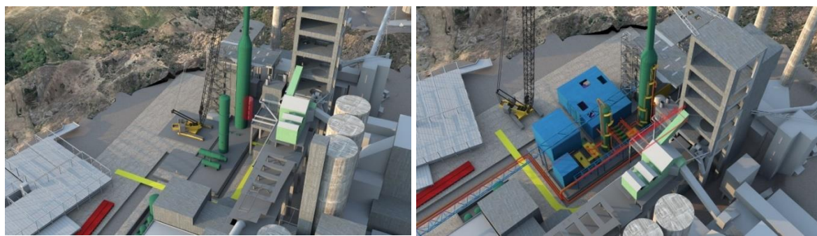
Figure 6-24: Location of crawler crane for lifting operations in the main process area
