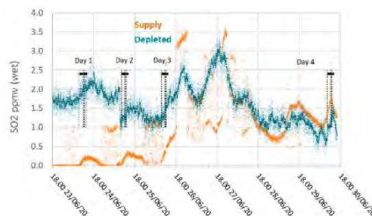
Figure 6: Supply and depleted flue gas SO 2 measurements throughout the test period
