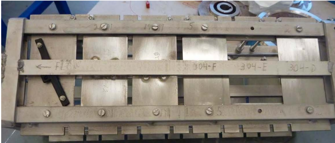
Figure 2: Illustration of coupons installed in the rack. Flow direction from right to left.
