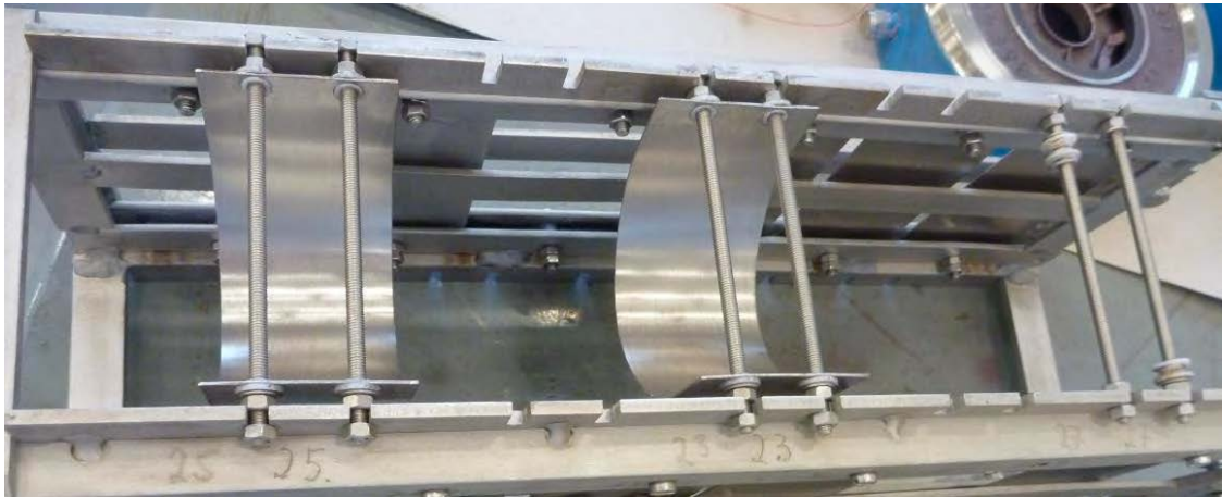
Figure 3: Illustration of bent coupons installed in the rack. Flow direction from right to left.
