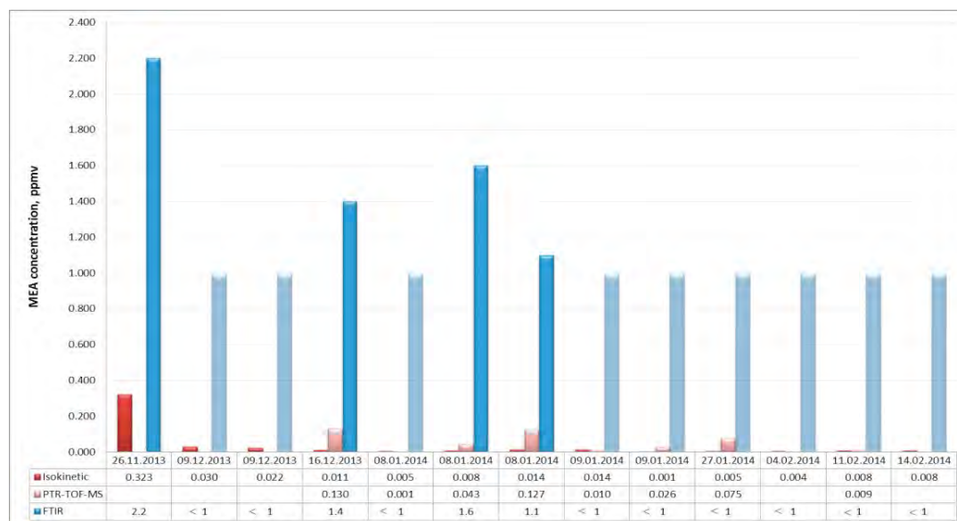
Figure 6: MEA emissions determined by different analyzer techniques during the campaign. Results on the FTIR below detection limit (<1 ppmv) are colored lighter blue.
