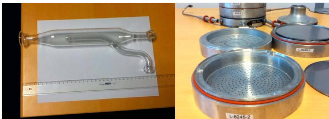
Fig. 3. Glassware that directs part of the incoming flow towards the impactor and an additional flow to match the sampling system to the probed conditions and operate under near-isokinetic sampling conditions (left). Demounted Anderson Cascade Impactor with 8 stages each containing a nozzle plate and a tray for aerosol collection (right).
