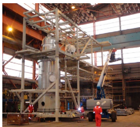
Figure 3 Picture of construction of one reboiler on a pre-assembled unit at the Aker Stord yard
