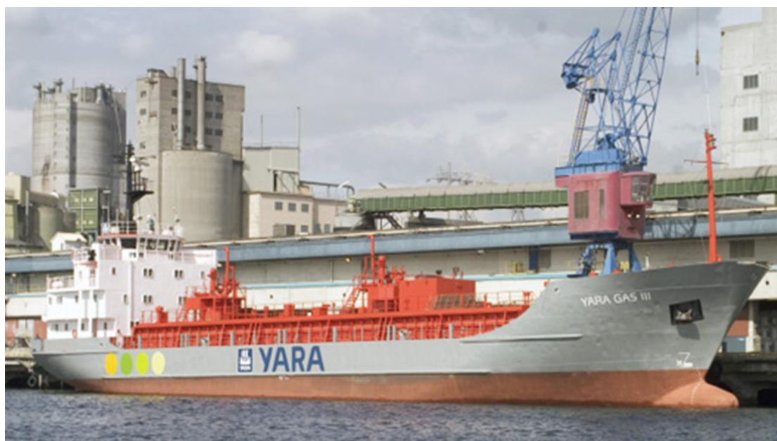
Figure 5. M/T Yara Gas III alongside the quay near Yara's ammonia plant in Porsgrunn (Capacity: 1200 t of liquefied CO 2 in 2 tanks of 600 tons capacity each. Ship type: Converted container vessel).
