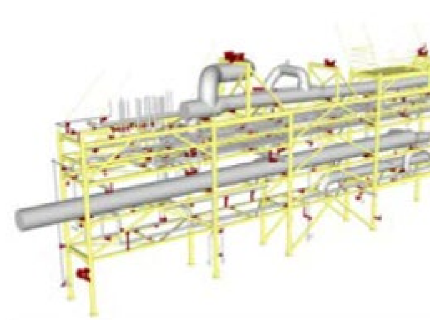
M02: Piperack 02 Lifting weight = 111T
