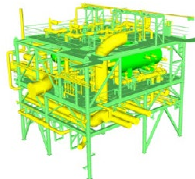
M03: Liquefaction Module Lifting weight = 212T
